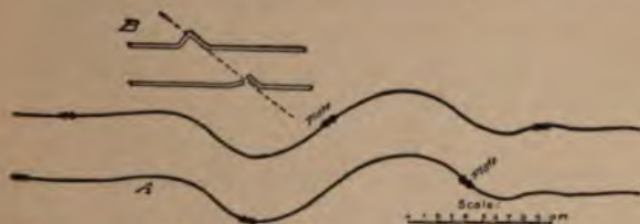
FIG. 64. — Diagrams to show how railway tracks are either broken or buckled locally within the district visited by an earthquake.
